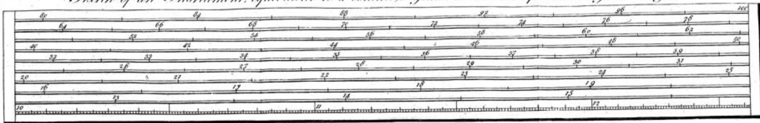
Sketch of an Instrument, equivalent to a common Gunter's Scale 20 feet in length. Fig. 1.
